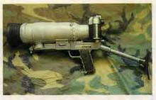
ABOVE: Left side of Soviet Photo-Sniper unit showing the assembled camera, lens, lens shade, pistol grip and buttstock. Note that name plate above pistol grip is in English. This is typical of Soviet equipment intended for export, since outside the Soviet Union more people are familiar with English than with Russian.
